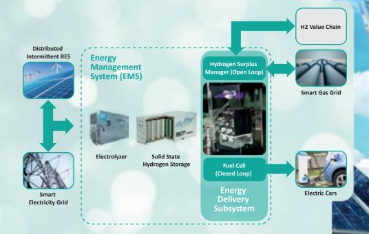
The INGRID project will be demonstrated through the design, deployment and the operation of a 39 MWh energy storage real life demonstrator located in Puglia, the Italian region with the largest RES portfolio. Such facility includes an hydrogen energy storage installation with more than 1 ton of safely stored hydrogen and a novel fast responding 1.2 MW electrolysis hydrogen generator and will provide smart balancing support for the local distribution power grid.
